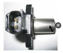
To fit the gasket (Rotax 431 500, thickness 0,8 mm) between the pick-up and the crankcase is an allowed option.
