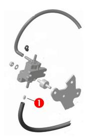
To fit the impulse nozzle **0** into the pressure hose is an allowed adjustment. The direction of the impulse nozzle inside the pressure hose is free.
